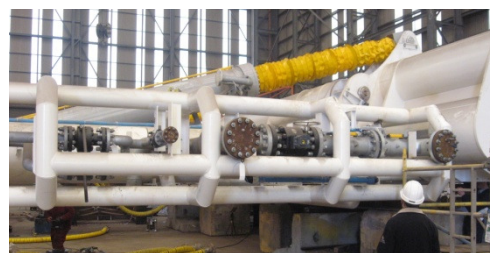
WEC Check Valves and Manifolds
